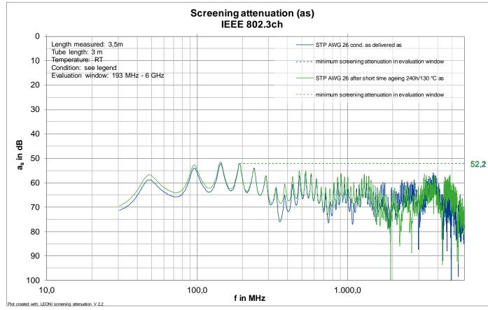
Condition as delivered and after short time ageing (240h/130°C) at room temperature.
