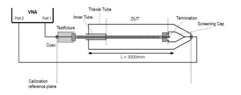
• The measured cables are bulk cable <u>without</u> any inliner or connector
