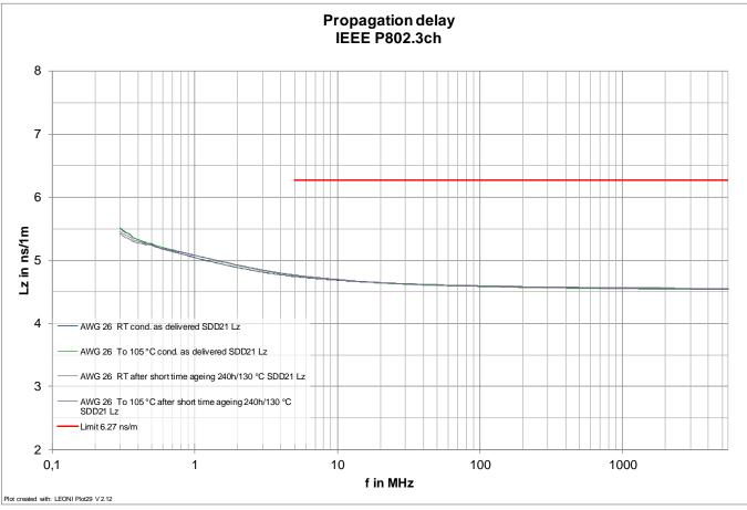
Propagation delay always better than the required 6,27 ns/m in all conditions.
