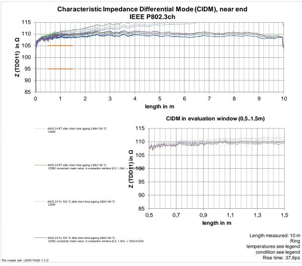
Impedance of AWG 24 PROTOTYPE needs more improvement which will lead to an increase of insertion loss (simulation data added to the insertion loss diagram).
