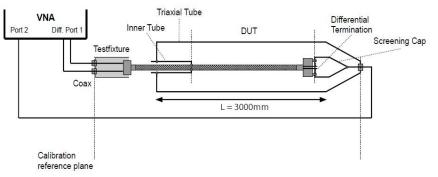
• The measured cables are bulk cable <u>without</u> any inliner or connector
