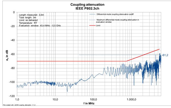
Condition as delivered (new) at room temperature
