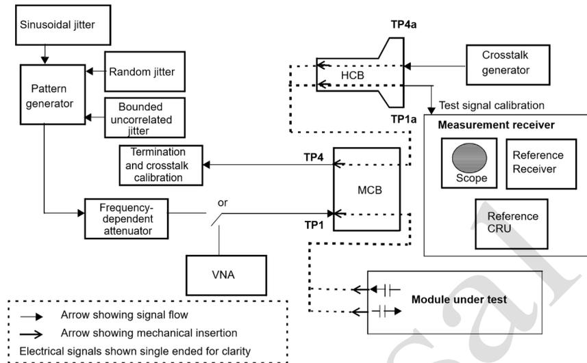
Figure 120G-10—Example module stressed input test setup
