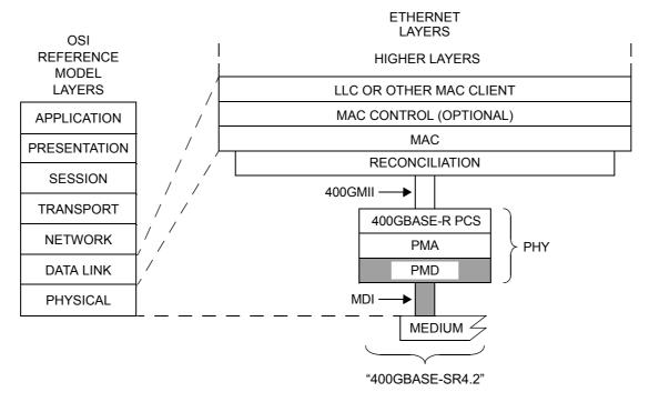
400GMII = 400 Gb/s MEDIA INDEPENDENT INTERFACE LLC = LOGICAL LINK CONTROL MAC = MEDIA ACCESS CONTROL MDI = MEDIUM DEPENDENT INTERFACE PCS = PHYSICAL CODING SUBLAYER PHY = PHYSICAL LAYER DEVICE PMA = PHYSICAL MEDIUM ATTACHMENT PMD = PHYSICAL MEDIUM DEPENDENT
