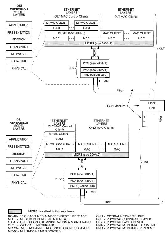
Figure 200A–2—Relationship of EPON P2MP PMD to the ISO/IEC OSI reference model and the IEEE 802.3 Ethernet model
