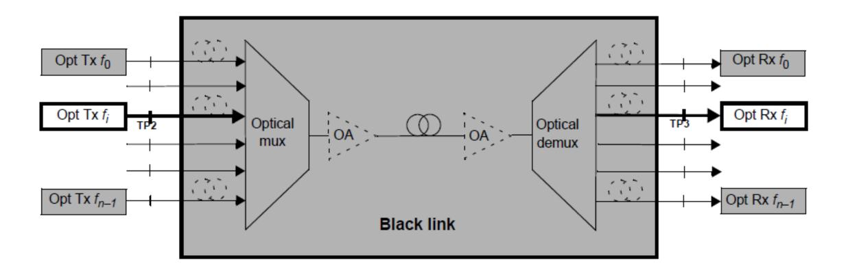
Fully consistent with Figure 5-1 in G.698.2. The transmitter frequency is used instead of transmitter wavelength, no OADM is shown, and "black link" is referred to instead of "DWDM link".
