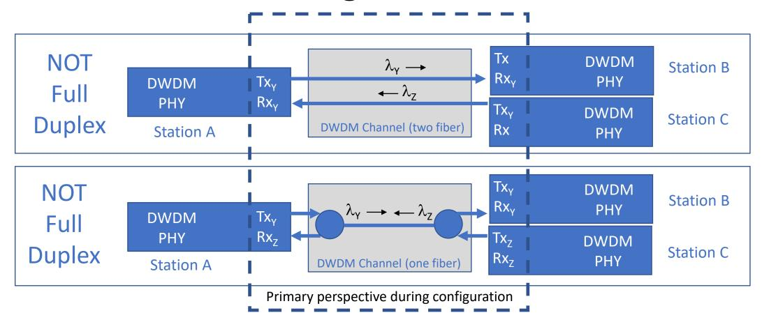
Not examples of full duplex operation as specified for 802.3 Ethernet (See Slide #3)
