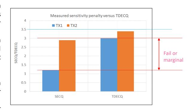
If TDECQ-SECQ will not be carefully quantified, what can then happen then is the absurd situation that after propagation tests a 'good' transmitter ends with lower TDECQ with respect a worse one, but just fails the new TDECQ-SECQ metric ...
