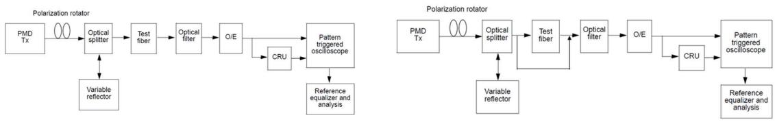
Figure 151-4—TDECQ conformance test block diagram
