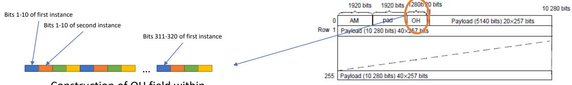
Construction of OH field within the 400GBASE-ZR frame
