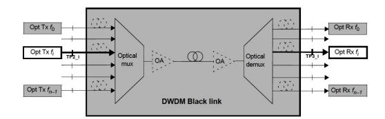
Figure 156-5—Black link example configuration for specifying n DWDM channels
