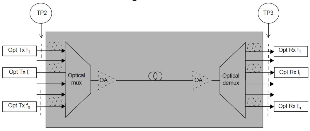
Figure 154–3—Example configuration of the black link approach
