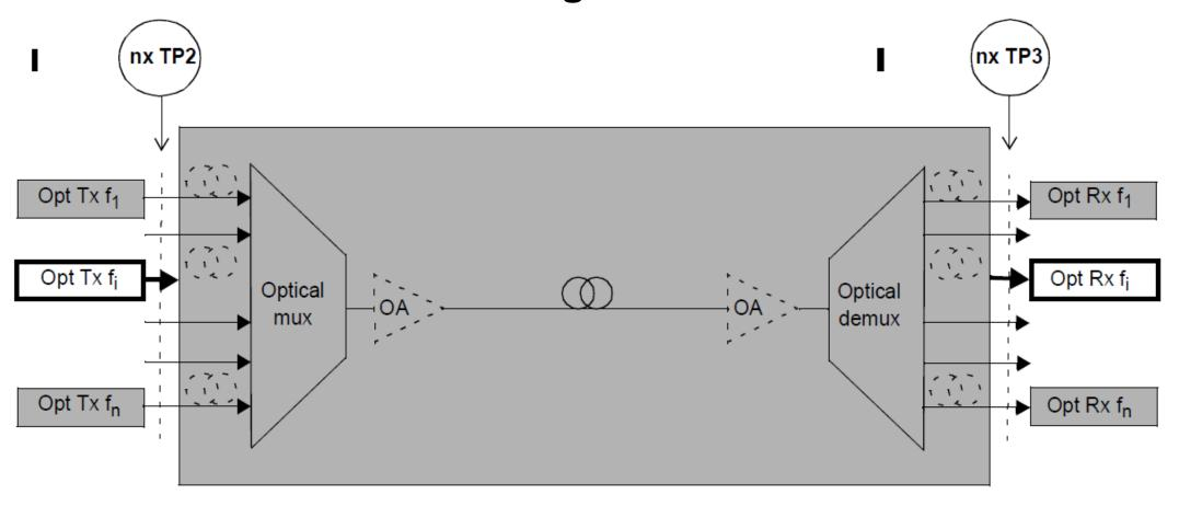
Figure 154–3—Black link example configuration for specifying n DWDM channels
