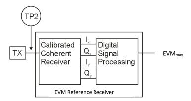
A block diagram for the EVM conformance test is shown in figure 156-7. Connect the 400 Gb/s DP-16QAM transmitter and calibrated coherent receiver using a single-mode fiber patch cord between 2 m and 5 m in length. The conformance test setup consists of the functional blocks described in 156.9.10.1.1 through 156.9.10.1.8. The EVM reference receiver is used for the measurement of  $EVM_{max}$ .
