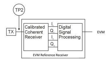
A block diagram for the EVM conformance test is shown in figure 156-7. Connect the 400 Gb/s DP-16QAM transmitter and calibrated coherent receiver using a single-mode fiber patch cord between 2 m and 5 m in length. The conformance test setup consists of the functional blocks described in 156.9.10.1.1 through 156.9.10.1.8. *Add text clarifying nature of EVM reference receiver*.
