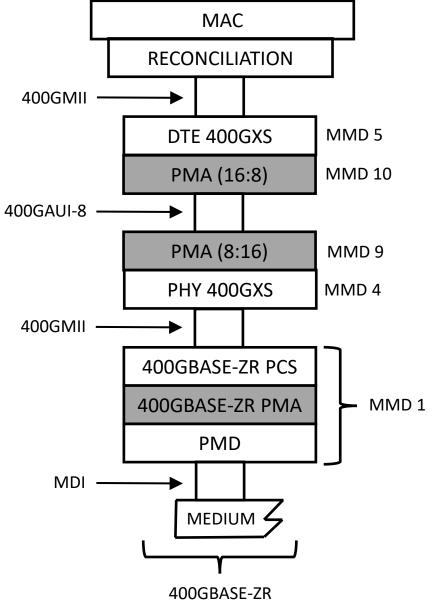
400GAUI = 400 Gb/s ATTACHMENT UNIT INTERFACE 400GMII = 400 Gb/s MEDIA INDEPENTENT INTERFACE 400GXS = 400 Gb/s EXTENDER SUBLAYER DTE = DATA TERMINAL EQUIPMENT MAC = MEDIA ACCESS CONTROL MDI = MEDIUM INDEPENDENT INTERFACE MMD = MDIO MANAGEABLE DEVICE PCS = PHYSICAL CODING SUBLAYER PMA = PHYSICAL MEDIUM ATTACHMENT PMD = PHYSICAL MEDIUM DEPENDENT
