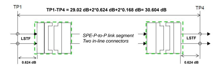
Link segment insertion loss at 7031.25 MHz
