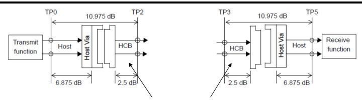
Host Compliance Board (TP2 or TP3) - Plug in at TP2 or TP3 for TX and RX
