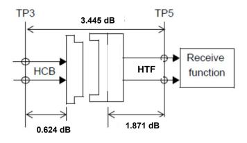
TP0-TP2=1.871 dB+0.624 dB +0.624 dB +0.168 dB +0.168 dB = 3.445 dB TP0-TP2=1.871 dB+0.624 dB +0.624 dB +0.168 dB = 3.445 dB
