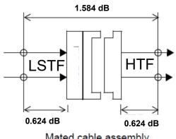
Mated cable assembly and test point test fixture
