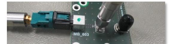
4. In-situ de-embedding removes fixtures 1 and fixture 2 from overall to get DUT as result
