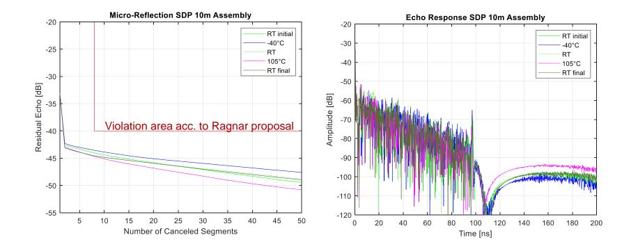
10 m cable assembly within the mask at all temperatures. Higher IL causes better results.
