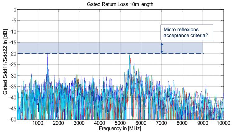
Modified procedure of Ragnar's micro reflexions analysis method is being investigated with results in frequency domain (return loss). Goal is to apply this method to whole channels.
