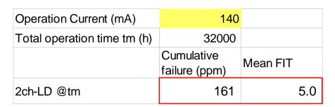
If=140mA 2ch-LD, Random=5Fit Cumulative failure rate: 161 ppm
