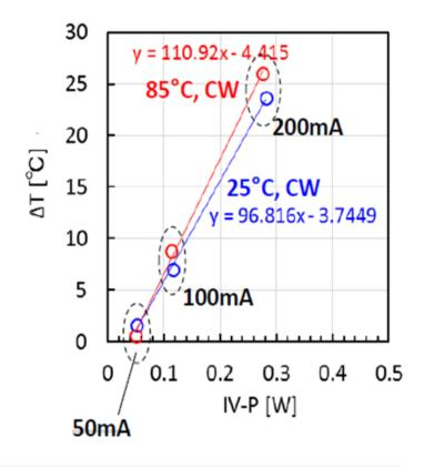
The temperature difference (ΔT) between Ta and Tj for Si-photonic modules is less than 20°C
