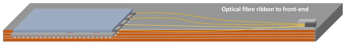
**High speed electrical PCB trace length range < 1 cm**
