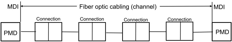
Note – The 50GBASE-AU power budget is based on 2 in-line connectors at 2.0 dB/connection. 4 in-line connections may be supported with lower loss connections.
