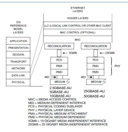
Relationship of 802.3cz PMDs to the ISO/IEC OSI reference model and the IEEE 802.3 Ethernet Model
