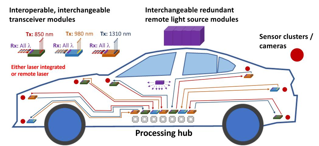
Interoperable PMD to serve automobile industry with multiple technologies for reliable automobile optical network. OEMs and suppliers can access optical technologies to test and select according to their requirements
