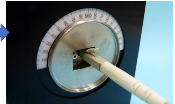
Milling fiber end with rotating cutting tool
