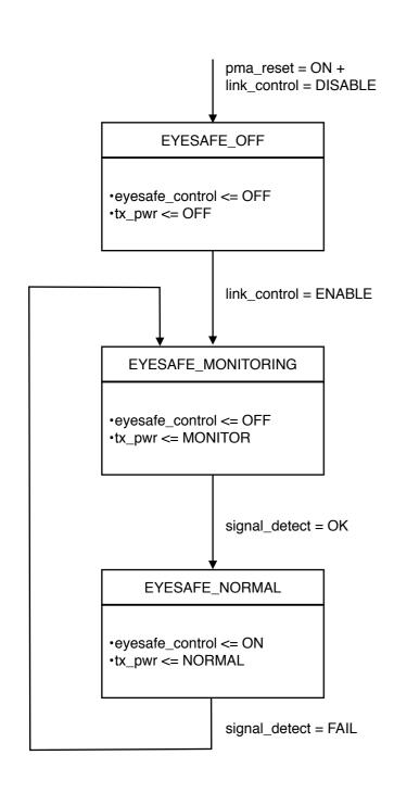
eyesafe\_control: variable set by the PMA eye safety control state diagram to control the operation of the PMA TX and RX.
