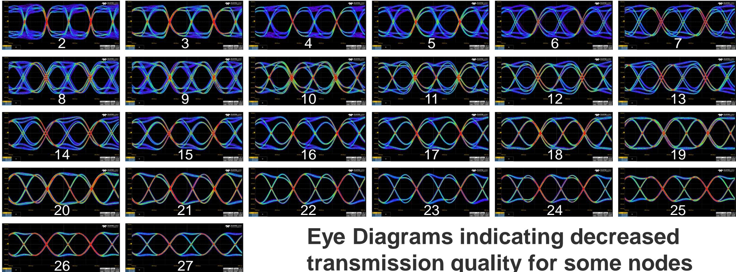
**Eye Diagrams indicating decreased transmission quality for some nodes due to massive overcompensation**
