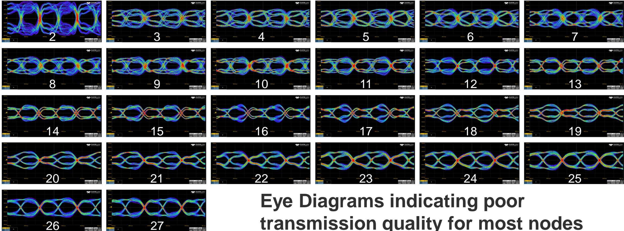
**Eye Diagrams indicating poor transmission quality for most nodes**
