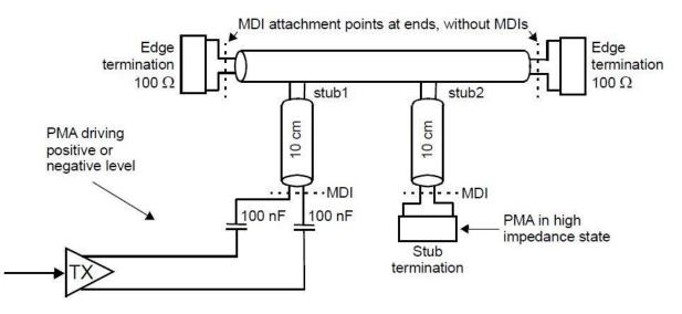
Figure 147–20—Multidrop line termination and PMA
