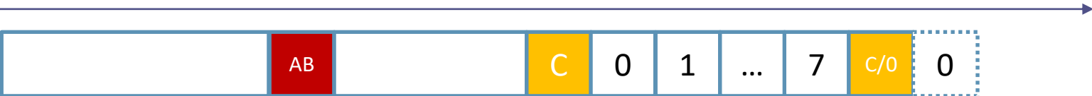
Ex 2: BEACONS from A and B collide, then A and B hear the BEACON from C and both renounce.
