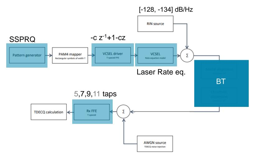
Utilized Bessel Thomson filters: -100m OM4: 15GHz -50m OM4: 21GHz
