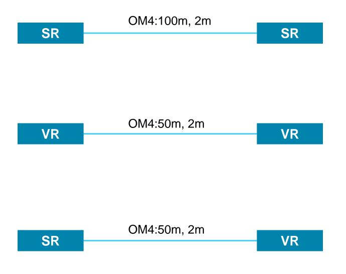
Some degree of Tx equalization is needed even for 25GHz VCSELs. The higher the pre-emphasis the better the eye for 100m but it can produce issues at 2 m (e.g, overshoot). Recommendation  $0.2 \le c \le 0.3$
