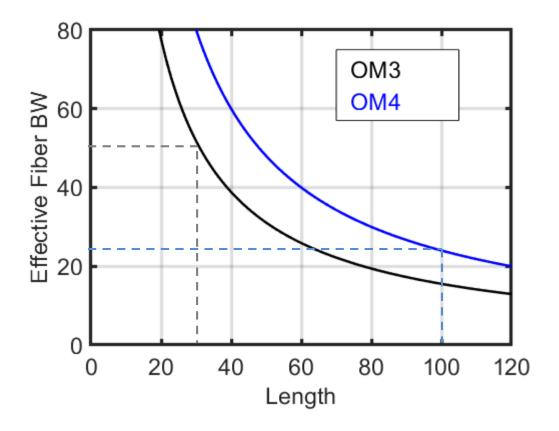
Effective fiber bandwidth calculated by adding modal and chromatic dispersion bandwidth in quadrature<sup>1,2,3</sup> at wavelength of 863 nm and RMS spectral width of 0.6 nm.
