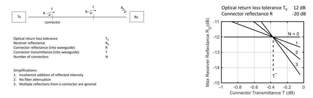
Conclusion: if the connector transmittance is at -0.37dB (a reasonable assumption), at 12dB ORL level, the ORL seen by TX doesn't depend on the number of connectors.
