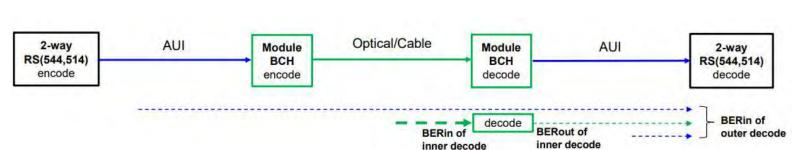
End to Segmented FEC as shown, for example, in welch\_3df\_logic\_220425.pdf
