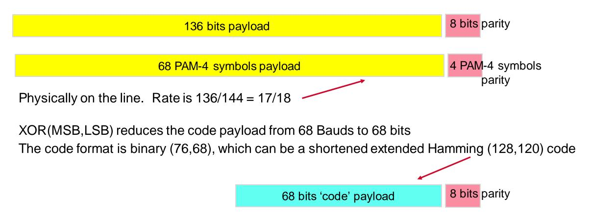
Decoding the shortened code points to the PAM-4 symbols to 'correct', which is unambiguous and essentially lossless compared to pointing to 'bits'
