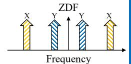
Physical picture:  $\Delta \phi(z) \sim 2\phi_y(z) - \phi_x(z)$  is fast varying (due to the very short fiber beat length of  $\sim 10$ m).
