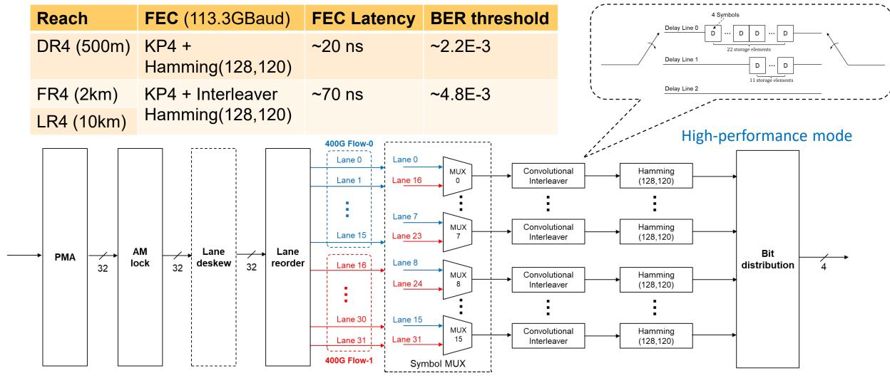
One ASIC to support High-performance or ultra-low latency mode by configurable interleaver.
