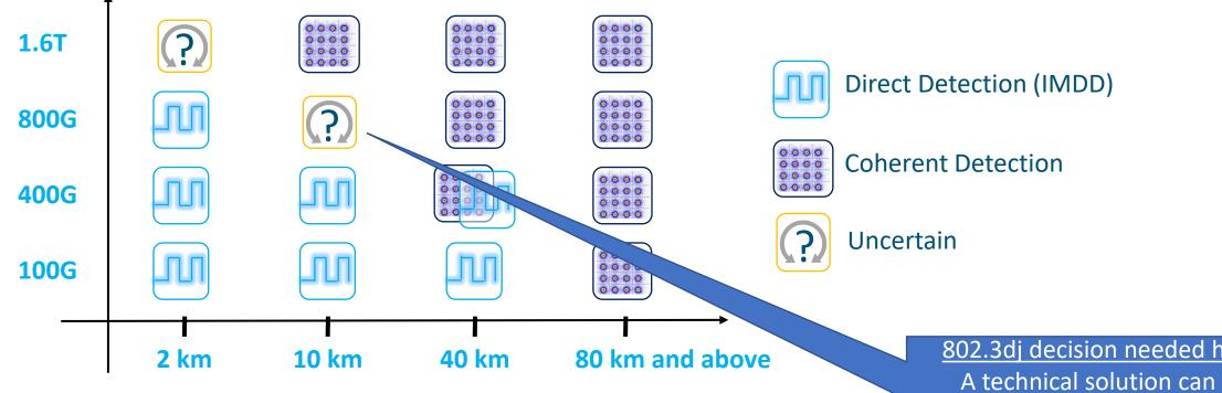
Duplex fiber solutions: As bit rate increases, longer reaches become more difficult. Creates a transition of technologies to keep up. 802.3dj decision needed here. A technical solution can be defined for both IMDD and Coherent. What will serve the needs of the user base better?
