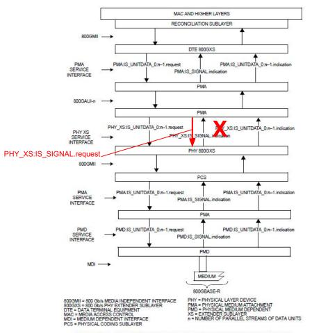
Figure 169–3—800GBASE-R inter-sublayer service interfaces including 800GMII Extender
