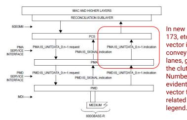
In new clauses 169. 173, etc., a parameter vector is used to convey a multitude of lanes, greatly reducing the clutter. Number of lanes is evident both due to the vector format and the related note in the
