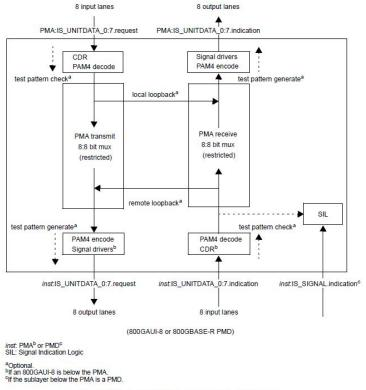
Figure 173-5-8:8 PMA Functional Block Diagram
