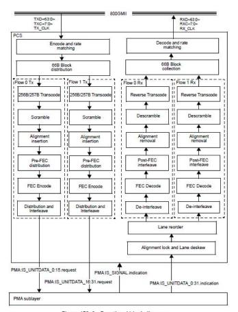
Figure 172-2—Functional block diagram
