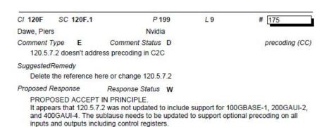
In 802.3ck, precoding capability was specified for 100GAUI-1, 200GAUI-2, and 400GAUI-4 (as shown by the last paragraph of 120F.1, below). 135.5.7.2 was updated to include 100GAUI-1, but 120.5.7.2 was not updated to specify this option for 200GAUI-2 and 400GAUI-4.
