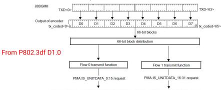
Figure 172-3-800GBASE-R PCS transmit bit ordering and distribution
