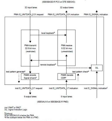
Figure 173-3-32:8 PMA Functional Block Diagram
