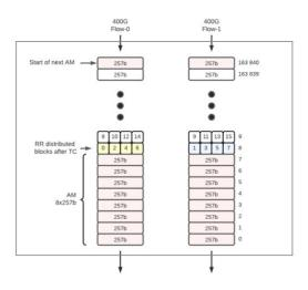
The transmit diagram in the baseline (slide 12) shows Alignment insertion as a single block across 2 flows.
