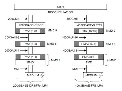
200GAUI = 200 Gb/s ATTACHMENT UNIT INTERFACE 200GMII = 200 Gb/s MEDIA INDEPENDENT INTERFACE 400GAUI = 400 Gb/s ATTACHMENT UNIT INTERFACE 400GMII = 400 Gb/s MEDIA INDEPENDENT INTERFACE MAC = MEDIA ACCESS CONTROL MDI = MEDIUM DEPENDENT INTERFACE MMD = MDIO MANAGEABLE DEVICE
