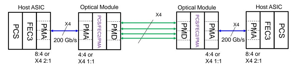
For scenario with 200 Gb/s per lane AUIs on both ends, same bit transparent mapping can be used in optical modules from FEC3 lanes to FEC2 operating in per-optical-lane style, similar to End-to-End scheme for breakout.
