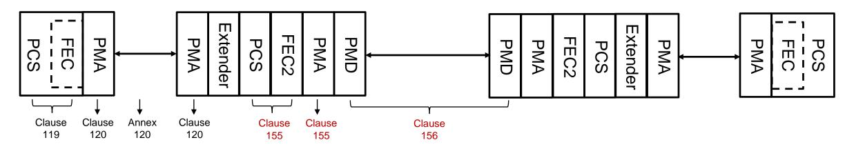
End-to-End scheme can translate to segmented by reusing PCS/FEC/PMA.
