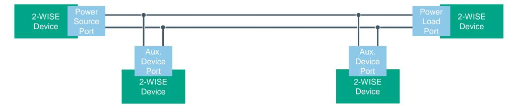
• 2-WISE system with auxiliary device ports (e.g. surge protection) connected via a series connection in the cable:
