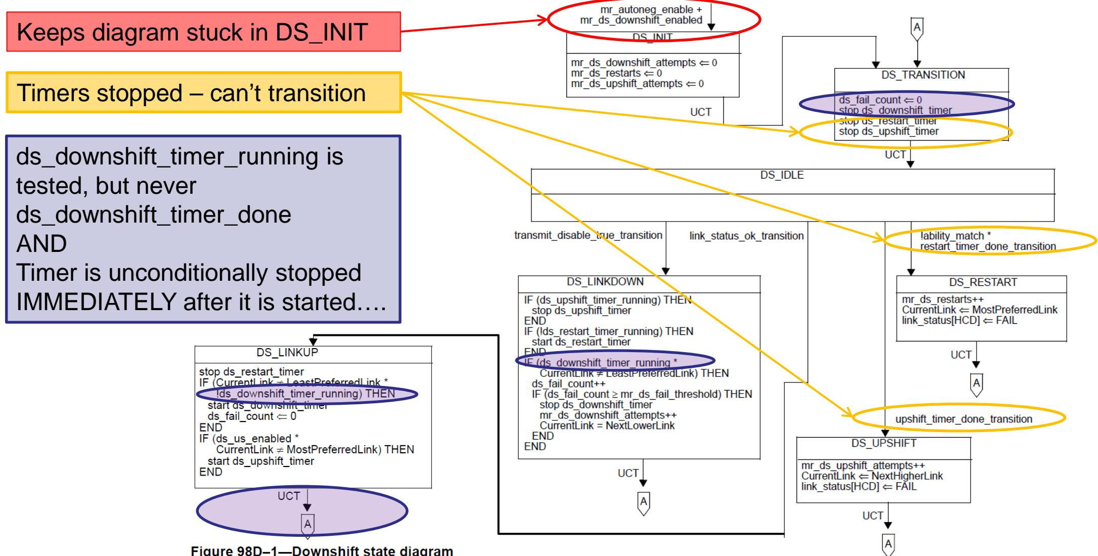
Figure 98D-1—Downshift state diagram
