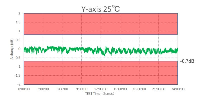
•The test results in the Y-axis were less than 0.5dB through the whole test.
