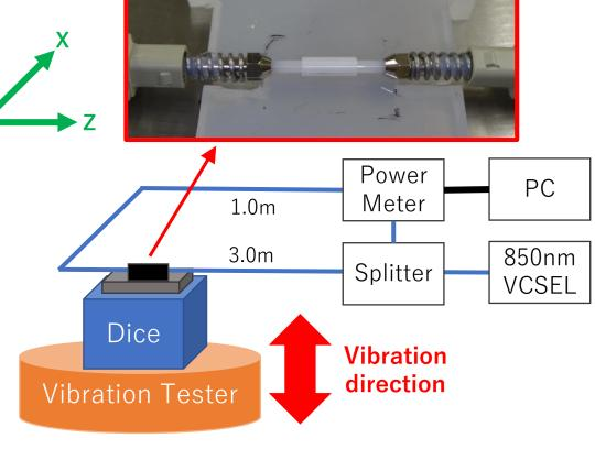
Fig 2, Schematic diagram of vibration test
