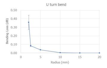
Low bending loss: less than 0.1 dB R=5mm
