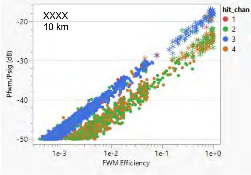
Using the equation  $P_{ijk}/P_s = \left(\frac{D_{ijk}}{3} \gamma L e\right)^2 \frac{P_i P_j P_k}{P_s} e^{-\alpha L \eta}$ , simplify the multi-variable Monte Carlo distribution to an equivalent single variable distribution with **Equivalent Launch Power**,  $P_{eq} = P_i = P_j = P_k = P_s$ ,  $\eta = 1$  and  $D_{ijk} = 6$  (non-degenerate):
