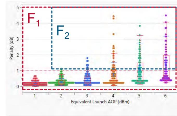
The fraction F<sub>1</sub> of links that have high FWM efficiency and power will experience high FWM penalties fraction F<sub>2</sub> of the time when using XYYX interleaving and fiber with PMD
