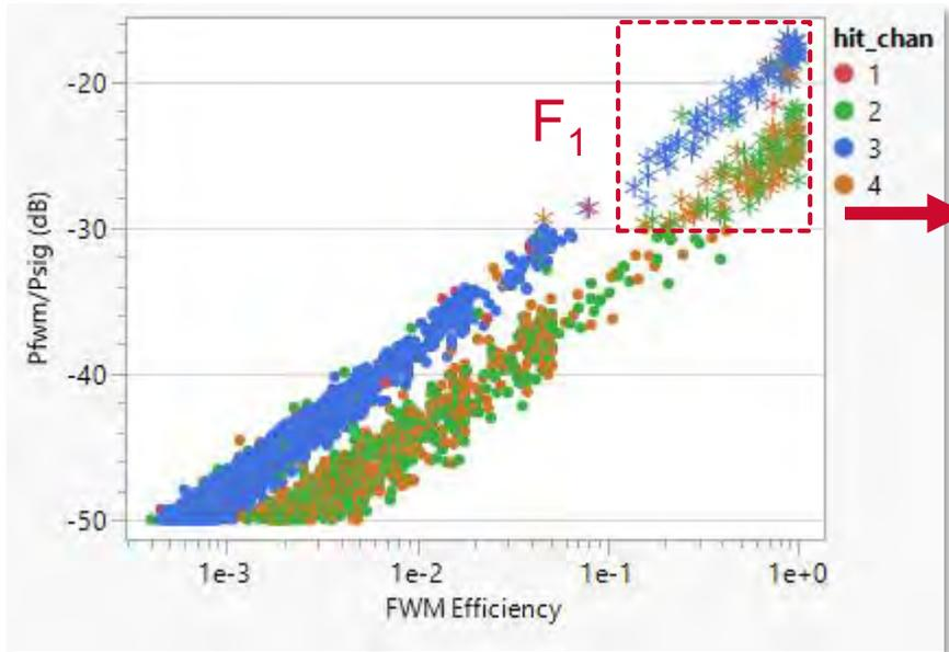
F<sub>1</sub> of channels have FWM efficiency and launch power high enough to cause an outage
