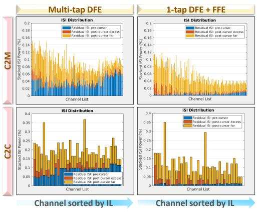
• Two receiver architectures are compared under the identical noise assumption and equalization length
