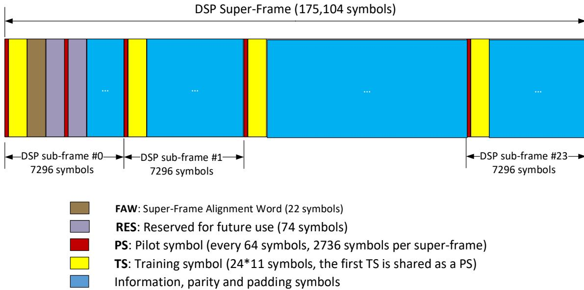
Pilot symbols shall be inserted every 64 symbols, starting with the first symbol of each DSP super-frame. The first 11 symbols of each DSP sub-frame can also be used for training (e.g, frame acquisition). The first symbol of the Training Sequence (TS) is a Pilot Symbol (PS).
