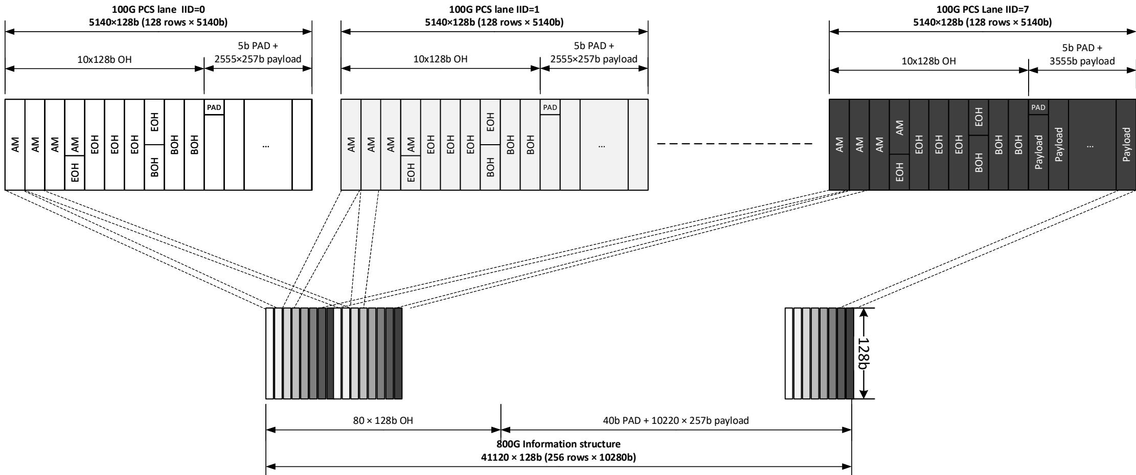
8 x 100G lanes are 128b interleaved to an 800G structure
