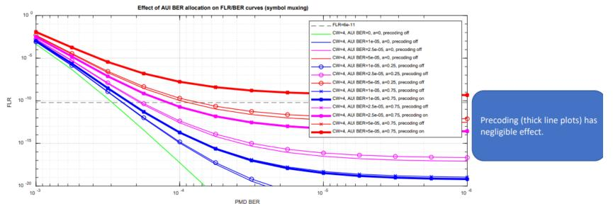
The blue curves are showing the effect of this error extension and also showing that the results with and without pre-coding are similar.
