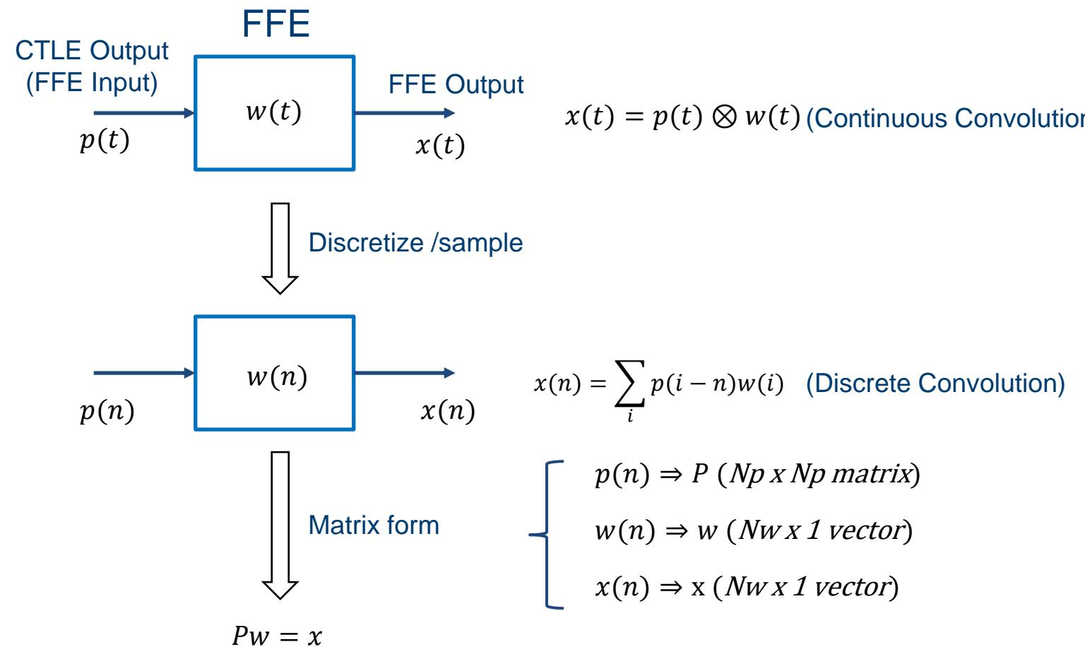
With the linear fitting (LF) method as in IEEE 802.3 Clause 85.8.3.3.5 and 85.8.3.3.6, we can determine FFE coefficients, i.e.  $h(n)$ , *with the following steps:*
