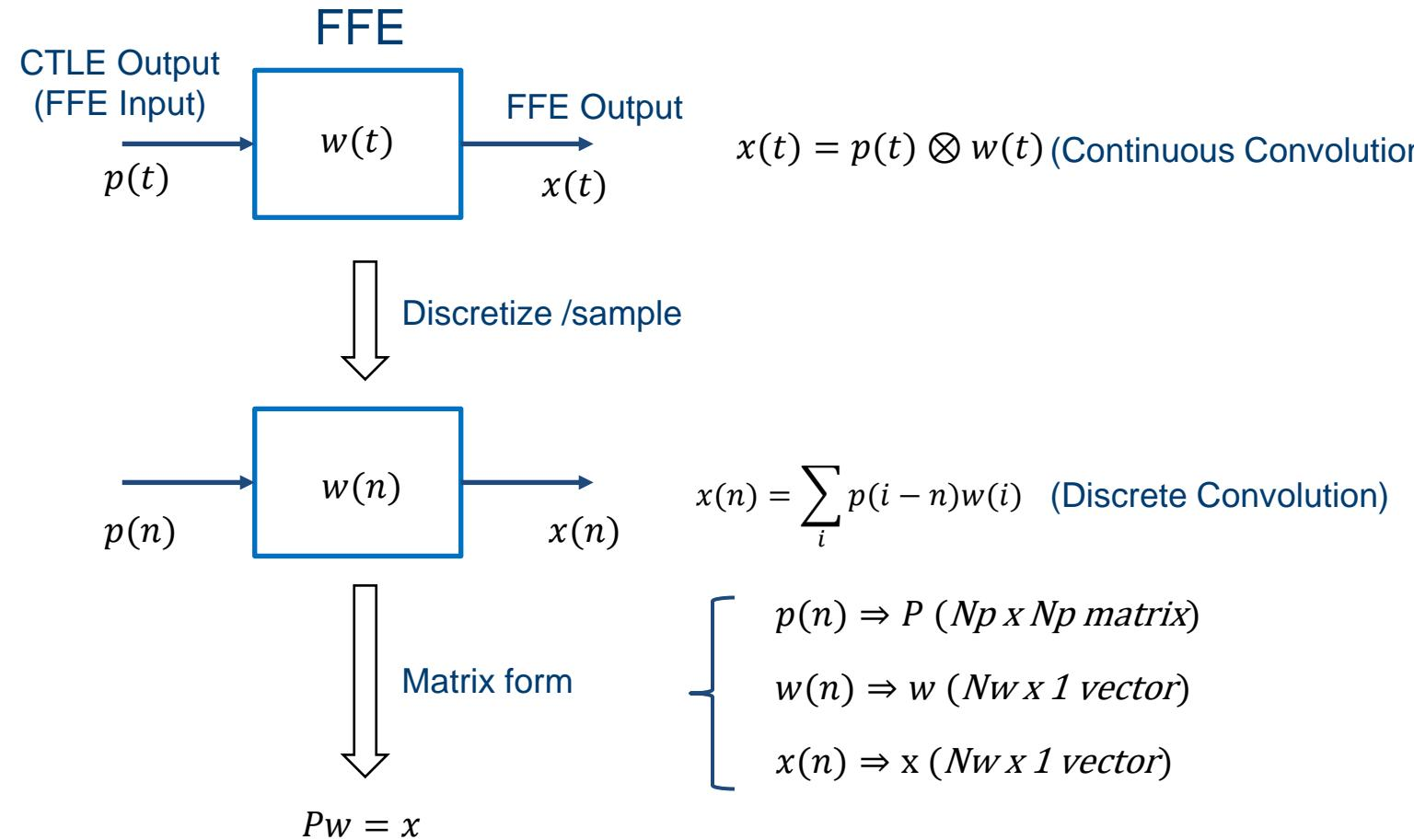
With the linear fitting (LF) method as in IEEE 802.3 Clause 85.8.3.3.5 and 85.8.3.3.6, we can determine FFE coefficients, i.e.  $w(n)$ , with the following steps:
