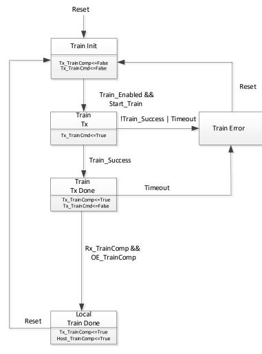
Tx\_TrainCmd = Tx\_TTS\_Control[5] Tx\_TrainComp = Tx\_TTS\_Status[6] OE\_Train\_comp= Rx\_TTS\_Status[6] Rx\_TrainComp <= Rx\_TTS\_Status[13] Host\_TrainComp = Tx\_TTS\_Status[15]
