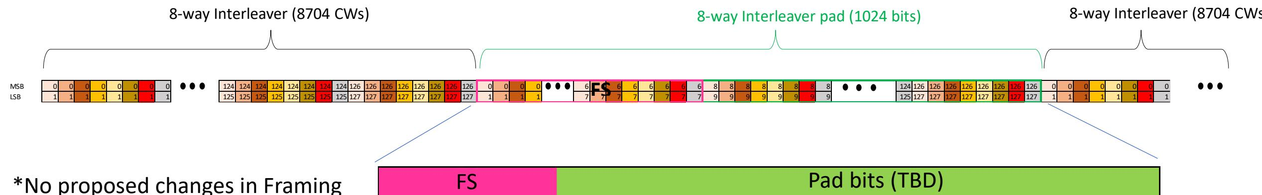
\*No proposed changes in Framing Sequence (FS) size (48 bit) and content on the PMA\_i lane
