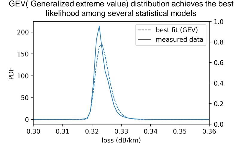
Insights: fiber loss has minima by nature, and GEV can both describe data maxima/minima and the distribution.
