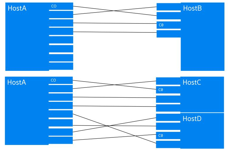
Need to resolve different understanding of lane "0" on both ends where Auto Neg can be performed
