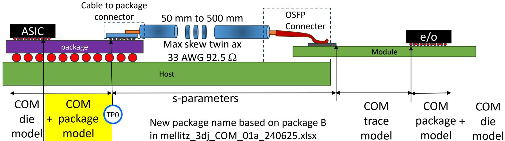
New package name based on package B in mellitz\_3dj\_COM\_01a\_240625.xlsx
