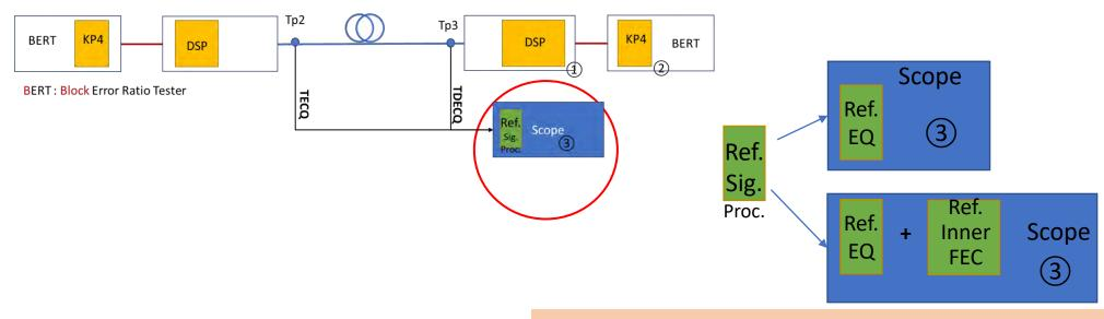
Both output an Eye Diagram which can be used for calculation of TDECQ Creating a universal measure for all 200G/L PMDs, Regardless of FECo/FECi
