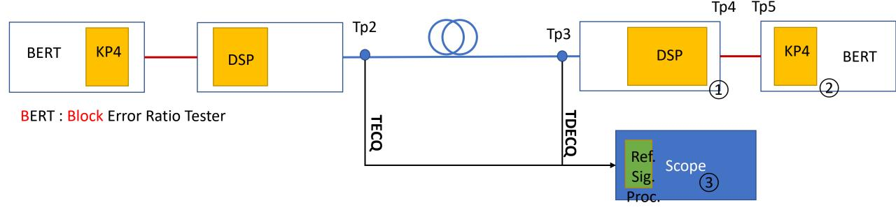
TP2 and TP3: not measuring error ratio, a PAM4 target SER ③ is used in the calculation of TECQ/TDECQ
