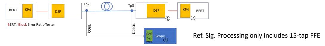
Build relation : 2x raw BER @ TP3/2 => 2x BER 1 = 2x f(Block Error Ratio 2)
